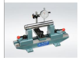
•Bench center can measure the workpiece without center hole, it can use for eccentricity and deflection of workpiece.
