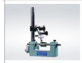
•Small bench center is suitable for measurement for small workpiece.
